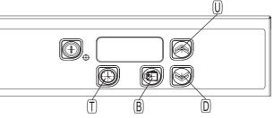
Select the parameter with the buttons "U"/"D" and press "B" to switch between label and value of the parameter; modify the parameter by pressing "U"/"D", then press the button "B" to confirm; wait 10 seconds to exit the parameter setting mode, or press the buttons "U"/"D" and "B" together
