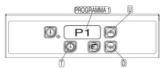
Press the button "T" again to select the programme number which is shown on the display, from P1 to P9.
